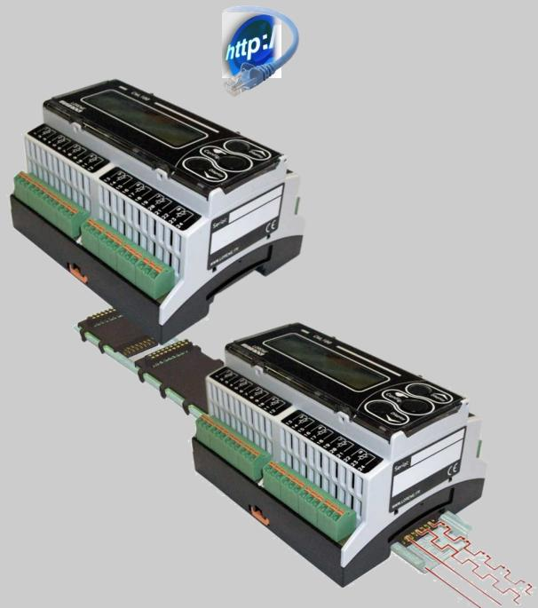
The Bus100 modular system provide an interconnection on Ethernet network, of different input / output and analogical acquiring module. The internal Bus (snap-on mounting on DIN rail) allow the connection of 12 modules. A "stand-alone" mode allows to an acquiring master module to drive directly an output relays module (local alarm).
